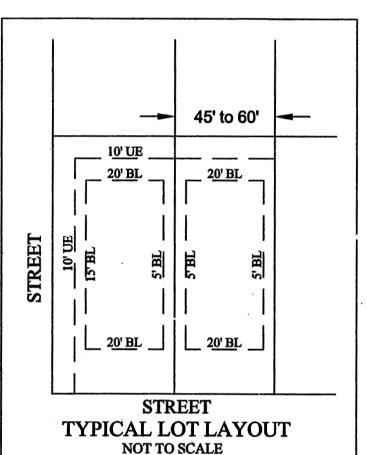
DRAINAGE EASEMENT NOTE: To allow for proper drainage conditions, all drainage easements shall be properly graded, maintained free and clear of obstructions, and special positive overflow sections (swales) shall be provided between lots which have an established FFE and shown hereon. Positive overthow sections (swales) shall be sloped to provide stormwater flow (i.e., drainage) from the front to rear of all lots affected hereon and will be maintained by the lot
