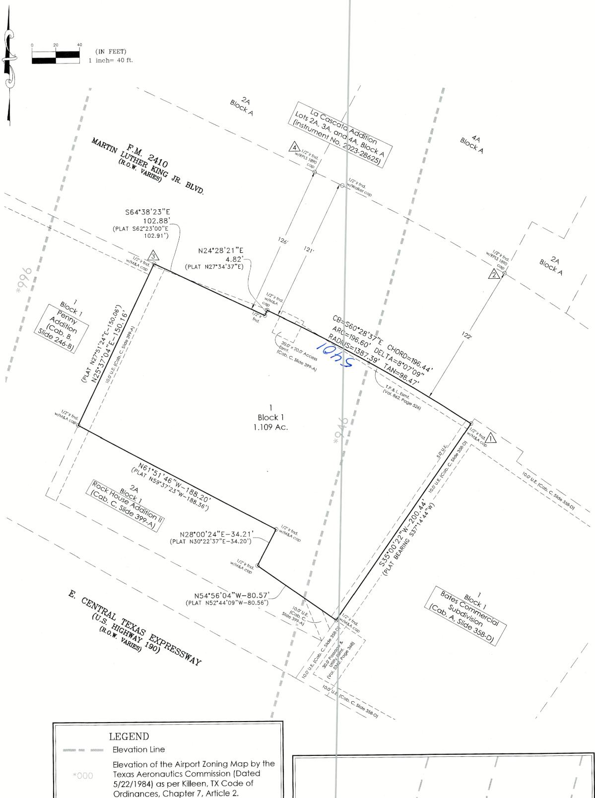
Bearings are based on the Texas Coordinate System, Central Zone, NAD 83 (CORS 96), as determined by Leica Texas SmartNet GPS observations.
